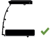
Make sure ladder is fully open before climbing up or down the ladder. Ladder should be against lower bunk profile.
