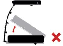
Lower bunk must be in down position before opening/closing ladder. Never attempt to raise lower bunk with the ladder in open position.
