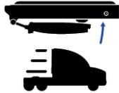
Make sure ladder is fully closed and in stowed away position while vehicle is in motion.
