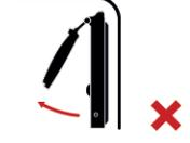
Do not unlock the ladder when the upper bunk is in stowed position.
