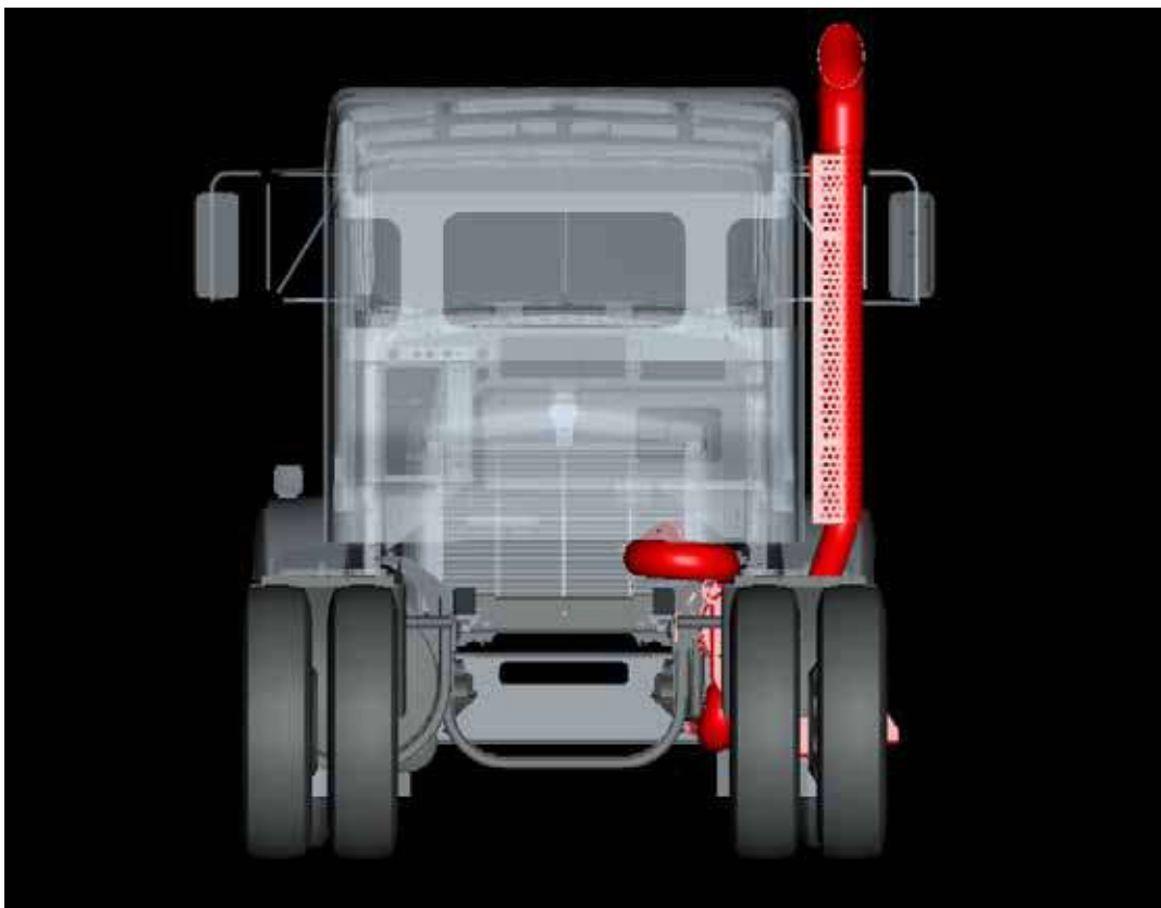
FIGURE 4-14: Back View of Right Hand Under DPF and SCR with Single SOC Tailpipe
