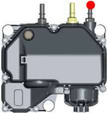
FIGURE 4-1: Measurement Location of DEF Supply Module (Pump)
