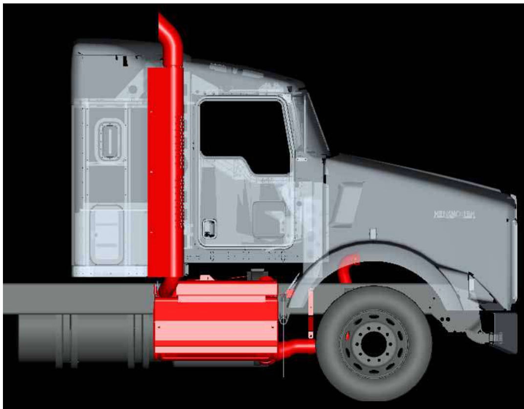
FIGURE 4-21: Right View of Right Hand Under DPF and SCR on Aerocab with Single SOC Tailpipe
