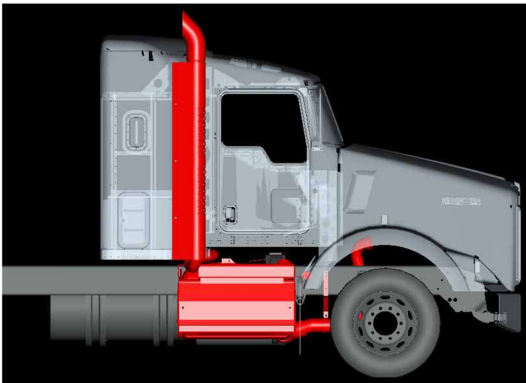
FIGURE 4-25: Right View of Right Hand Under DPF and SCR on Aerocab with Dual SOC Tailpipes
