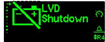
Low Voltage Disconnect
