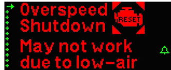
Engine Over-Speed Shutdown Low Air Warning
