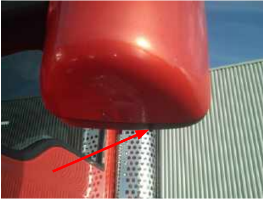
FIGURE 2-3: Aerodynamic Mirror OAT Sensor Location
