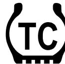
Watches vehicle's wheel speeds to detect slippage and may reduce engine power, or apply vehicle brakes, to help regain traction.
