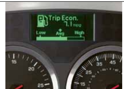
Kenworth's multi-function Drive Performance Center provides the driver with important real-time information on truck performance. The touch of a button displays up-to-the-second readouts on cumulative trip fuel economy, optimum RPM for maximizing fuel efficiency, and system diagnostics (in language a lay person can understand). Comprehensive truck specification data – unique to the vehicle – is also available to speed troubleshooting and parts replacement.
