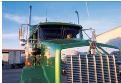
A sloped hood gives the driver a much better view – offering more in-front-of-the-truck visibility than straight hood conventionals.
