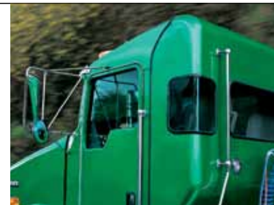
Optional cab corner windows help drivers who need to see better in reverse, at intersections and around the job site.
