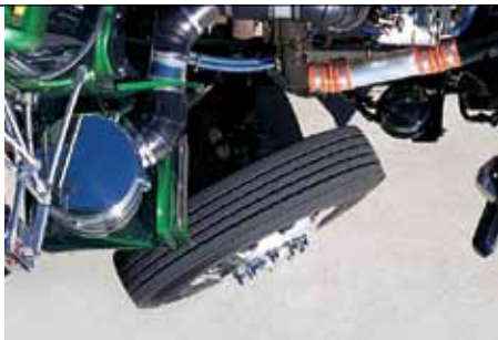
The T800's set-back front axle – together with steering geometry that delivers up to 54 degrees of wheel cut – helps drivers optimize and maneuver loads with ease.
